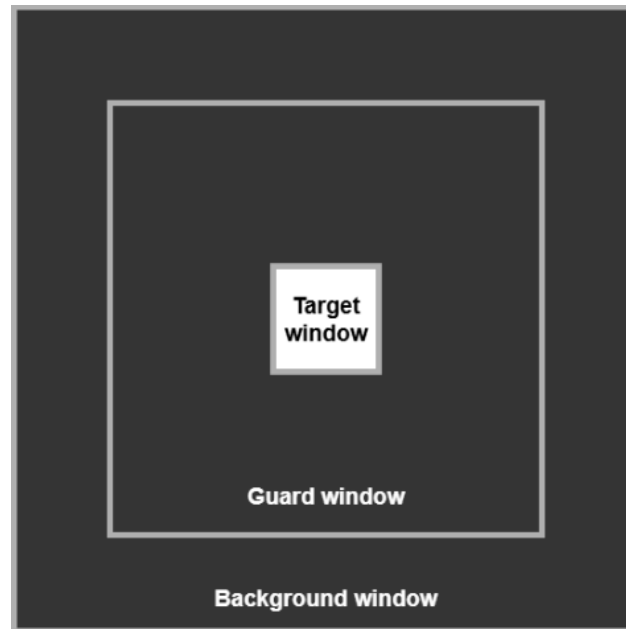
Figure 1. The concept of the Adaptive threshold algorithm as a base for the Ship Detection workflow
