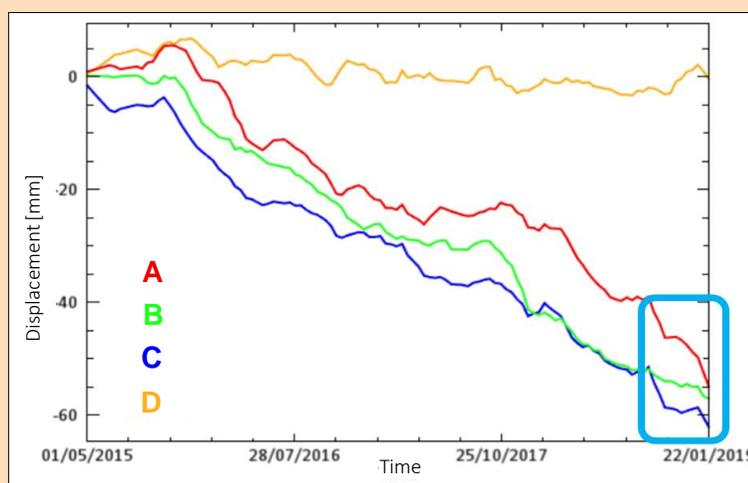
A first analysis based on the annual average velocity displacements inferred from Sentinel-1 data acquired from May 2015 to January 2019 – as illustrated in the figure on the top – reveals significant movements not only for the collapsed dam – marked with the red square – but for most of the other tailing dams within an area of around 120 km<sup>2</sup>.
