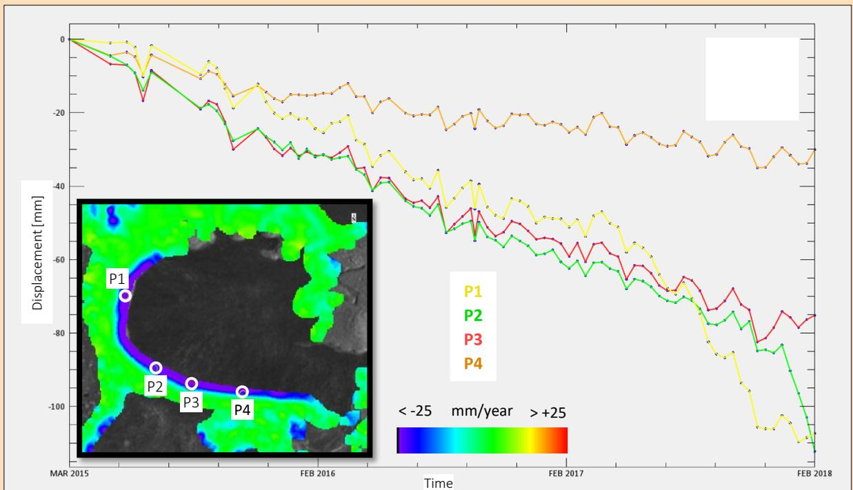
This analysis does not pretend to provide an interpretation of these phenomena, since the risk management needs to be investigated by structural engineers. However, since the deformation process has been active over the whole observation period, it appears unlikely that the earthquake could be identified as the only or major cause of the collapse.
